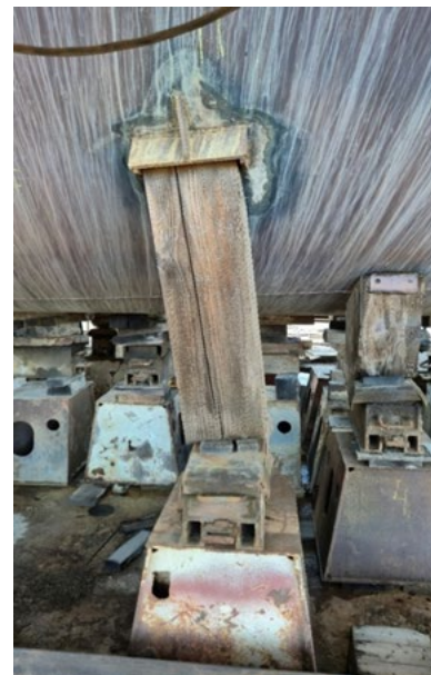
Pomaci upornih elemenata uslijed zastoja gradnje / Shift of support blocks under the vessel due to an extended construction downtime
