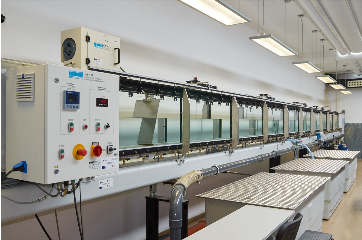
Figure 5.1: Experimental flume as part of the hydraulic laboratory at the University of Rijeka.
