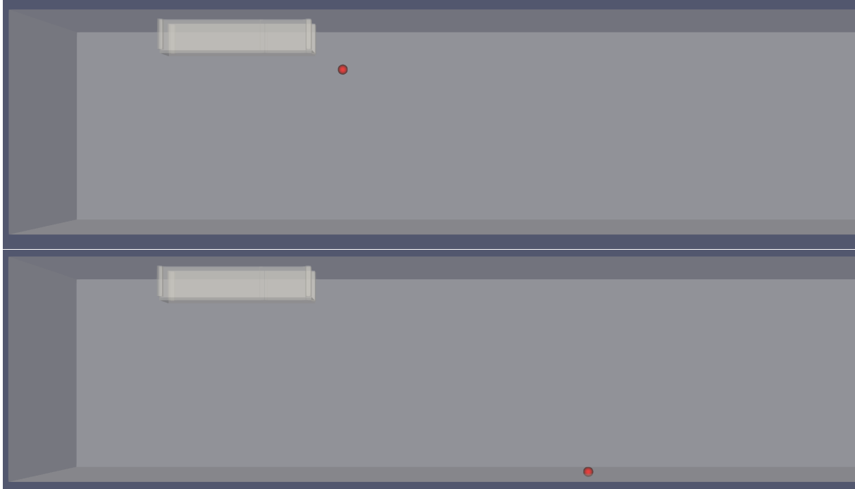
Figure 6.4: Example of numerical simulation for spherical particle settling in experimental flume (MP particle is marked with red dot). Upper picture represents particle in water stream while bottom one represents settled particle
