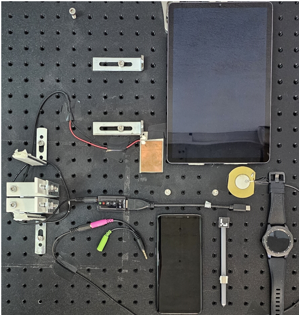
Figure 3.1: The experimental setup depicting all devices and sensors, including a tablet, a smartphone, a smartwatch, and two external piezoelectric sensors.
