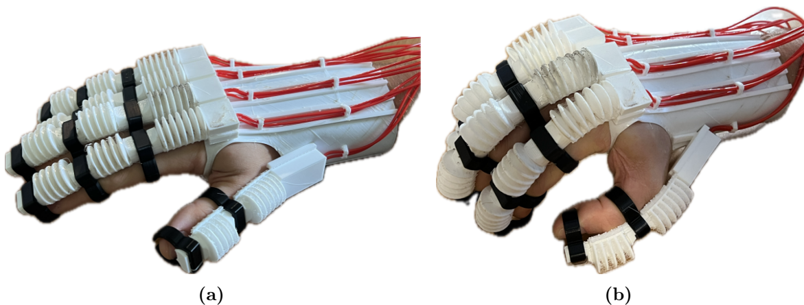
Figure 4.16 Soft-robotic glove fitted to the user's hand: (a) all SPAs in the initial position and (b) all SPAs activated.
