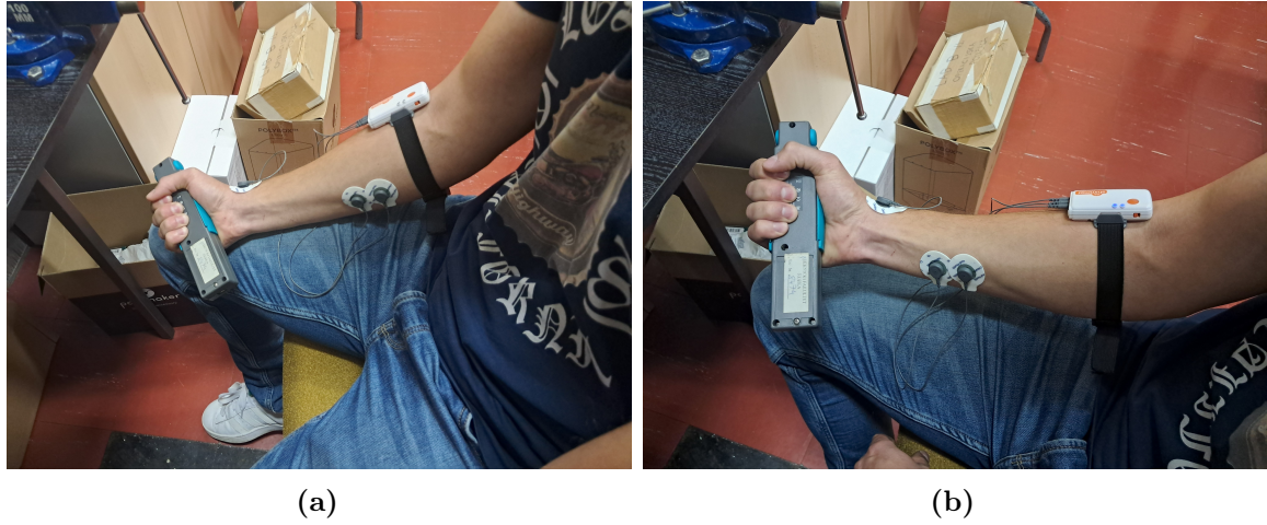
Figure 2.1 Placement of sEMG electrodes near flexor carpi ulnaris muscle on the forearm: (a) Position 1 (P1) and (b) Position 2 (P2).
