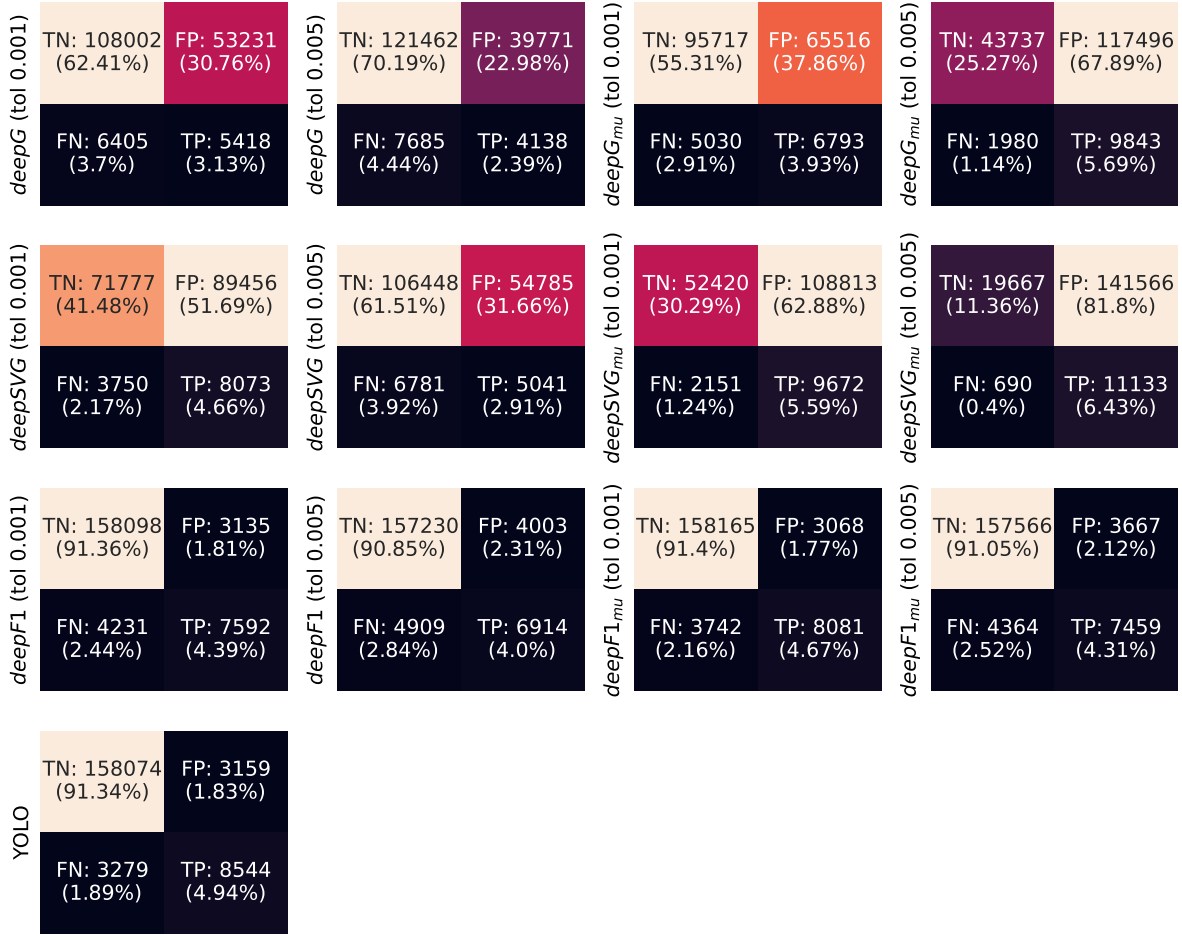
Figure 6.2: A confusion matrix heatmap with the average count and percentage of TP, TN, FP, and FN pixel classifications for the YOLO model [59] and the proposed models [178] on the underwater image dataset [143].
