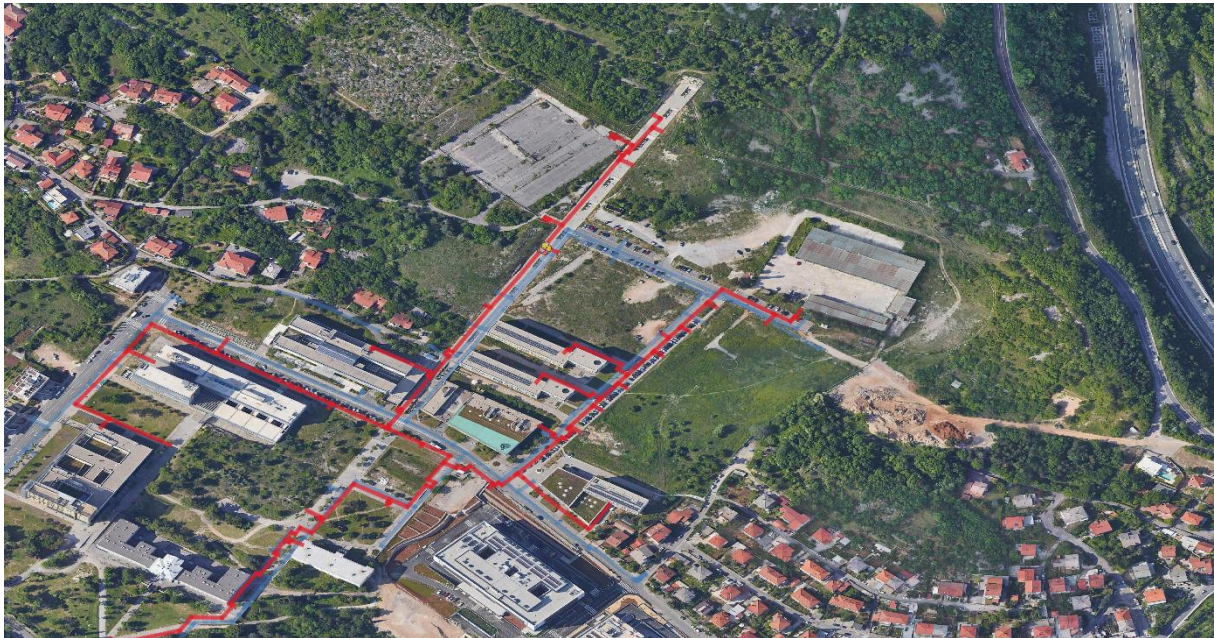
Figure 2.9 Pipeline positions of the district heating system (red) and water supply (blue) within a wider area, visualized using QGIS software and Google Maps.
