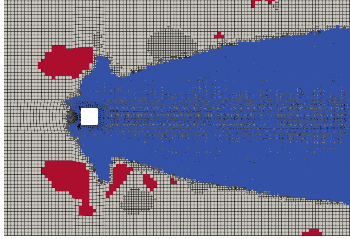
Figure 6.12: Regions of influence for refinement criteria in the square cylinder test case with AMR at the final time step. Blue indicates \Phi_{\lambda_2} , red indicates \Phi_{\Delta} .
