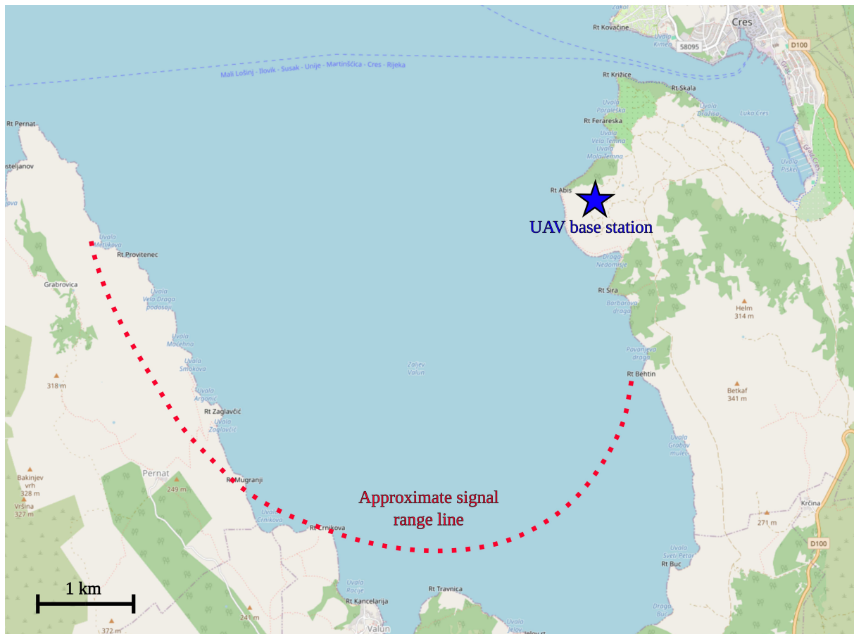
Figure 13.4: Observed UAV signal range during the Valun Bay sea surface search experiment.
