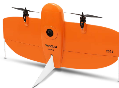
Figure 3.3: WingtraOne hybrid VTOL UAV [90].
