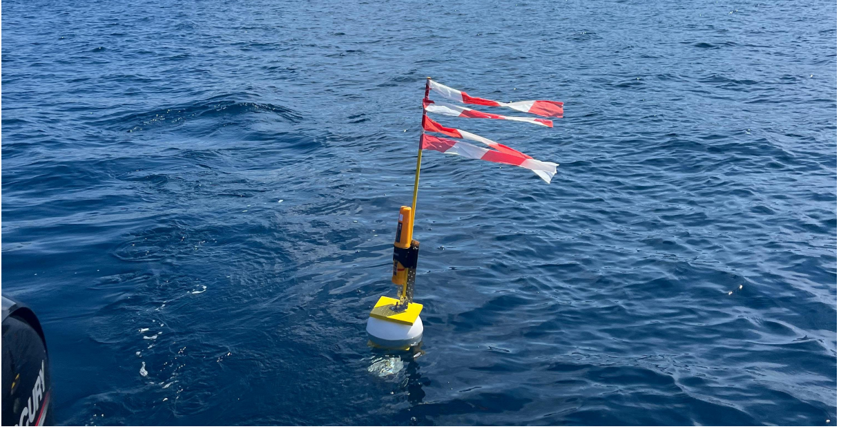
Figure 12.1: Deployed drifter used in the experiment for obtaining surface flow velocity measurements.
