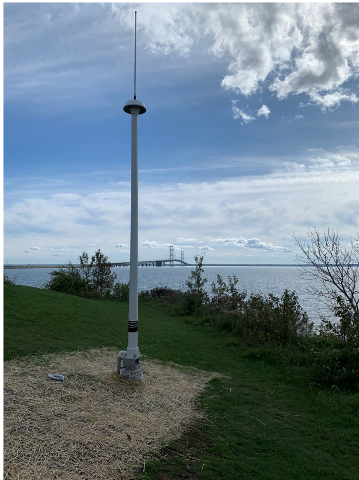
Figure 3.3: Great Lakes Observing System HF radar providing live snapshots of lake surface currents, 24 hours a day [97].
