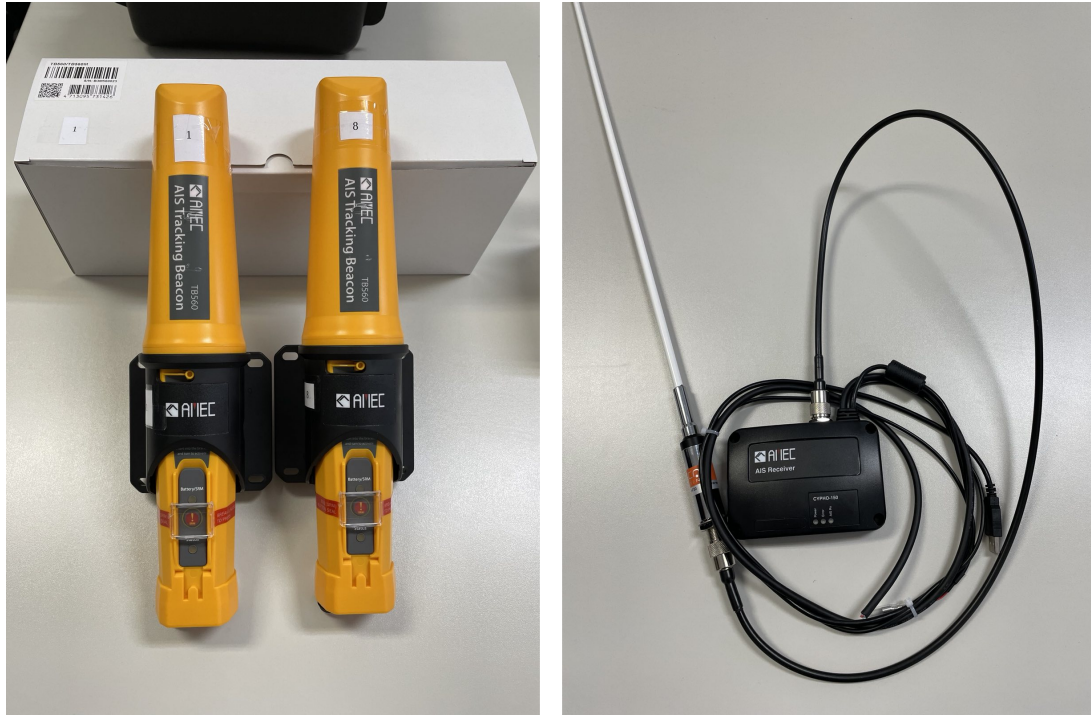
Figure 9.1: Labeled AMEC TB-560 tracking beacons (left) and AMEC Cypho-150 AIS receiver with VHF antenna (right), used for receiving AIS transmissions.
